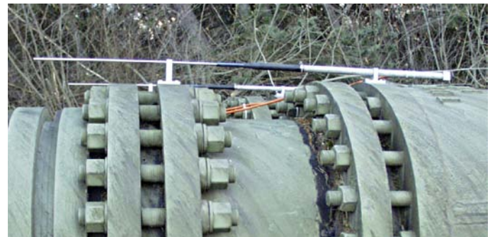
... to measure linear displacements in earth dams, at slopes and rocks or at pressure pipes and so on
