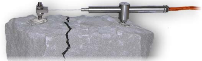
... to measure movements of joints, cracks and rocks as well as of rod extensometers
